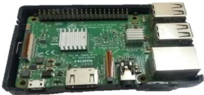
Gambar 1. Raspberry pi model b
